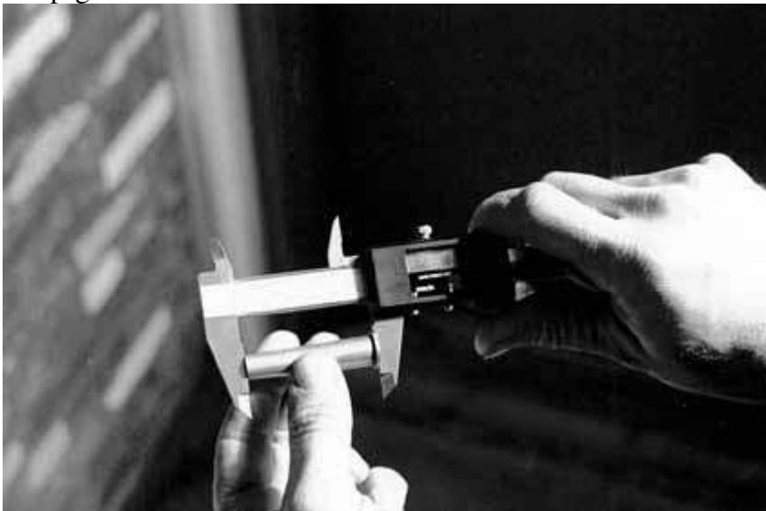
Through trial and error you can arrive at the proper seating depth. By inserting a bullet into an empty cartridge case you can chamber the round and then look and see where the rifling is engraving the driving bands. With the aid of a black magic marker to color the driving bands and a good magnifying glass, you will be able to better determine how far off the rifling you are seating your bullet. If the bullet is seated too far in or too far out,
