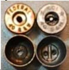
US. This photo shows two examples of 40S&W cases. The two cases on the left are Boxer-primed. Note the single concentric flash hole and the absence of an anvil. The Boxer anvil is an integral part of the primer -- not a part of the case. The two cases on the right are Berdan-primed. Note the concentric anvil located between two flash holes in the upper right. The Berdan primer has no integral anvil -- the Berdan anvil is an integral part of the case.
