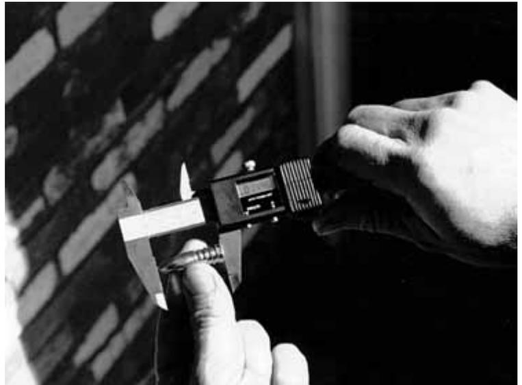
*Checking the overall length of a bullet.*
