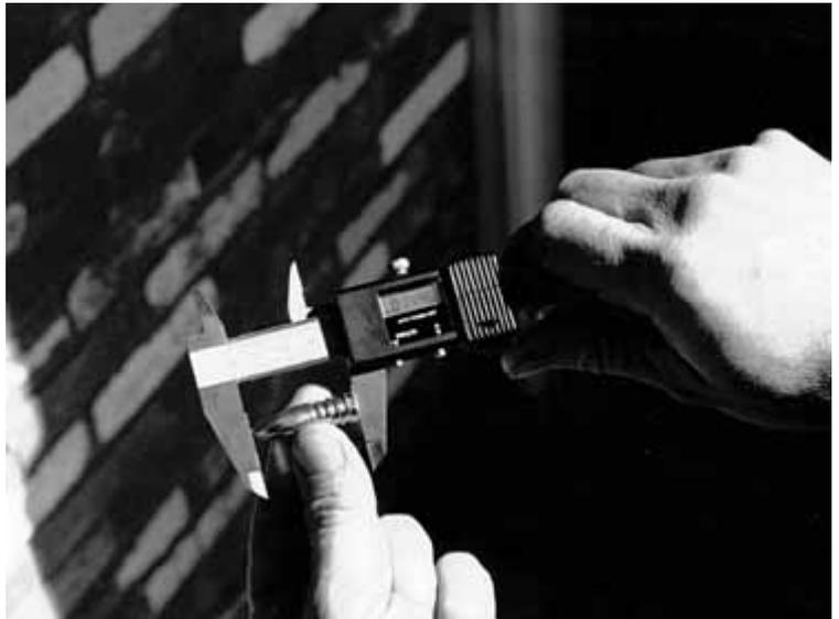
*Checking the overall length of a bullet.*
