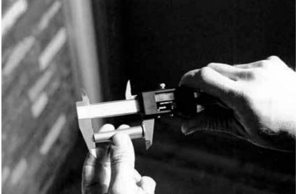
can arrive at the proper seating depth. By inserting a bullet into an empty cartridge case you can chamber the round and then look and see where the rifling is engraving the driving bands. With the aid of a black magic marker to color the driving bands and a good magnifying glass, you will be able to better determine how far off the rifling you are seating your bullet. If the bullet is seated too far in or too far out.
