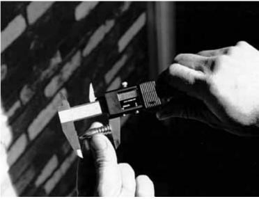
Checking the overall length of a bullet.
